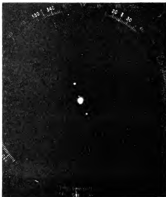
FIGURE 28 Comparison between blip intensities of ships and icebergs. Top radar scope photograph shows an iceberg (010°T; 18 200 yds) and a merchant ship, SS Mormacpena (047°T; 19,000 yds) on the 20-mile range scale. Bottom photograph compares a large iceberg (150°T; 7,000 yds) with the USNS Albatross (311°T; 6 000 yds).
